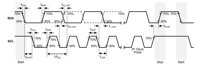
Figure 1. I<sup>2</sup>C Compatible Interface Timing
