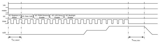
Figure 3. Enable of KTZ8868 via PWM
