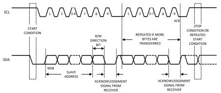
Figure 5. Data Transfer on I<sup>2</sup>C Serial Bus
