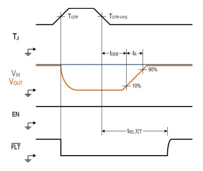
Figure 3. OTP Timing Diagram
