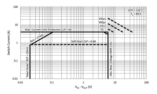
Figure 7. Safe Operating Area (SOA) for  $T_c = 80^{\circ}C$
