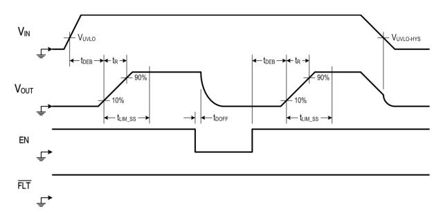
Figure 1. UVLO, Soft-Start and Turn-Off Timing Diagram
