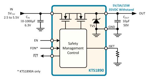
Figure 4. Functional Block Diagram
