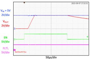
Over-Load Soft-Start & Auto-Retry Response (FON = low, Cout = 10μF, RLOAD = 1.5Ω)
