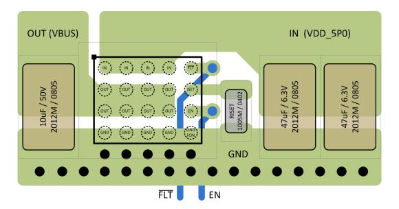
Figure 6. Recommended PCB Layout
