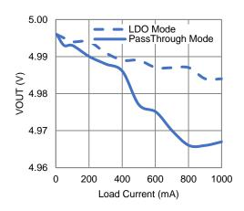
BPP, VOUT = 5V, 0 to 1A Load Transient
