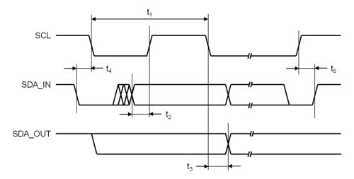
Figure 1. I<sup>2</sup>C Compatible Interface Timing Diagram
