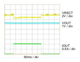
BPP, VOUT = 5V, Startup With 1A Load
