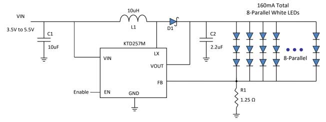
Figure 2. Application Circuit for 24 LEDs at 160mA Total Current (3-Series, 8-Parallel)
