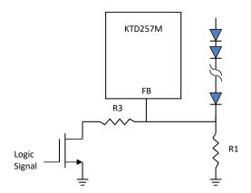
Figure 7. Dimming Control using a Logic Signal
