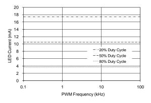
Figure 5. RC Filtered PWM Dimming Linearity (1kHz)
