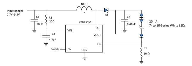
Figure 8. Application Circuit with Input RC Filter (required for 7- to 10-Series LED configuration)
