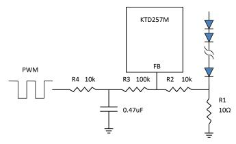
Figure 4. Dimming Control using an RC Filtered PWM Signal
