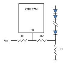
Figure 3. Dimming Control using a DC voltage
