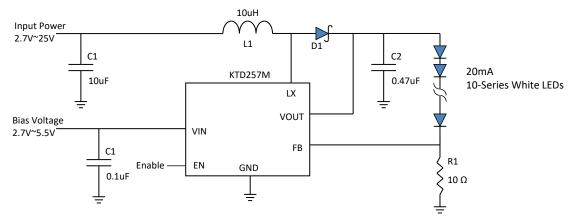
Figure 1. Application Circuit for 10 LEDs in Series with 20mA Current (VIN can be tied to input power rail if less than 5.5V)
