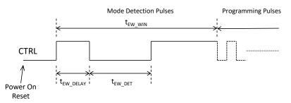
Figure 1. Dimming Mode Selection Pulses
