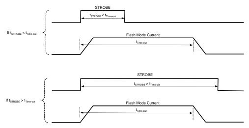
Figure 3. Flash Mode Current Controlled by STROBE (Edge Triggered)
