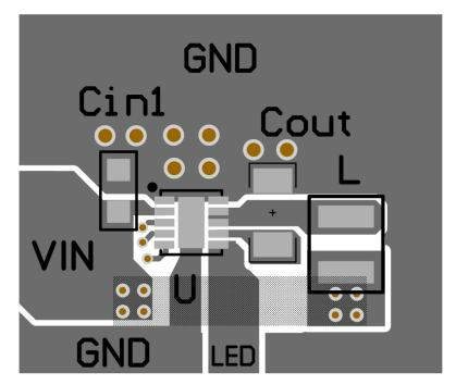
Figure 9. UDFN Recommended PCB Layout
