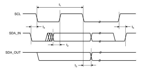
Figure 1. I<sup>2</sup>C Compatible Interface Timing
