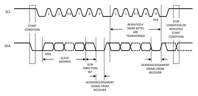
Figure 5. Data Transfer on I<sup>2</sup>C Serial Bus
