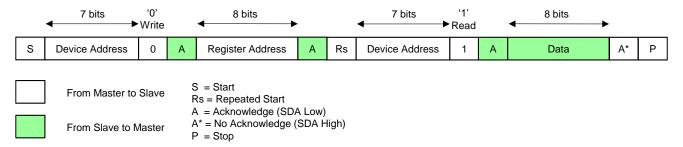
Figure 7. I<sup>2</sup>C Read Cycle
