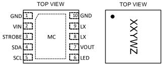
10-Lead 2mm x 2mm x 0.55mm UDFN Package **Top Mark**
