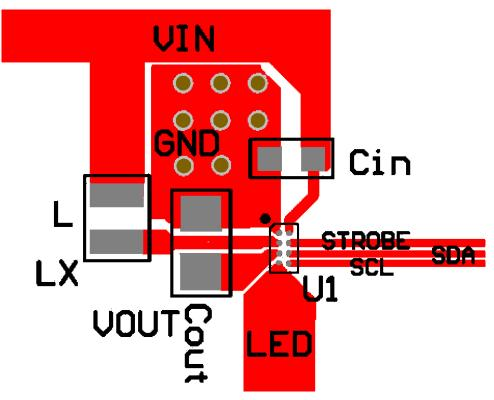
Figure 8. WLCSP Recommended PCB Layout
