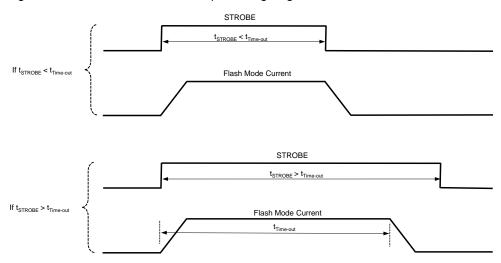
Figure 2. Flash Mode Current Controlled by STROBE (Level Triggered)
