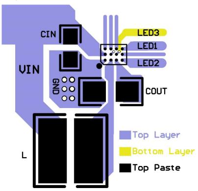
Figure 9. CSP Recommended PCB Layout
