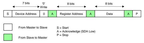
Figure 7. I<sup>2</sup>C Write Cycle
