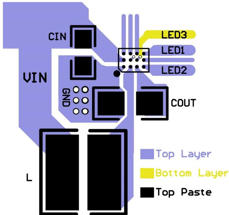
Figure 9. CSP Recommended PCB Layout
