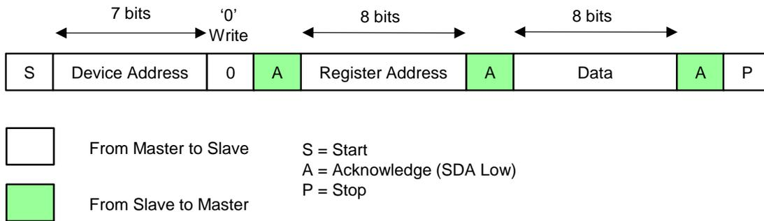
**Figure 7. I<sup>2</sup>C Write Cycle**
