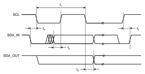
Figure 1. I<sup>2</sup>C Compatible Interface Timing
