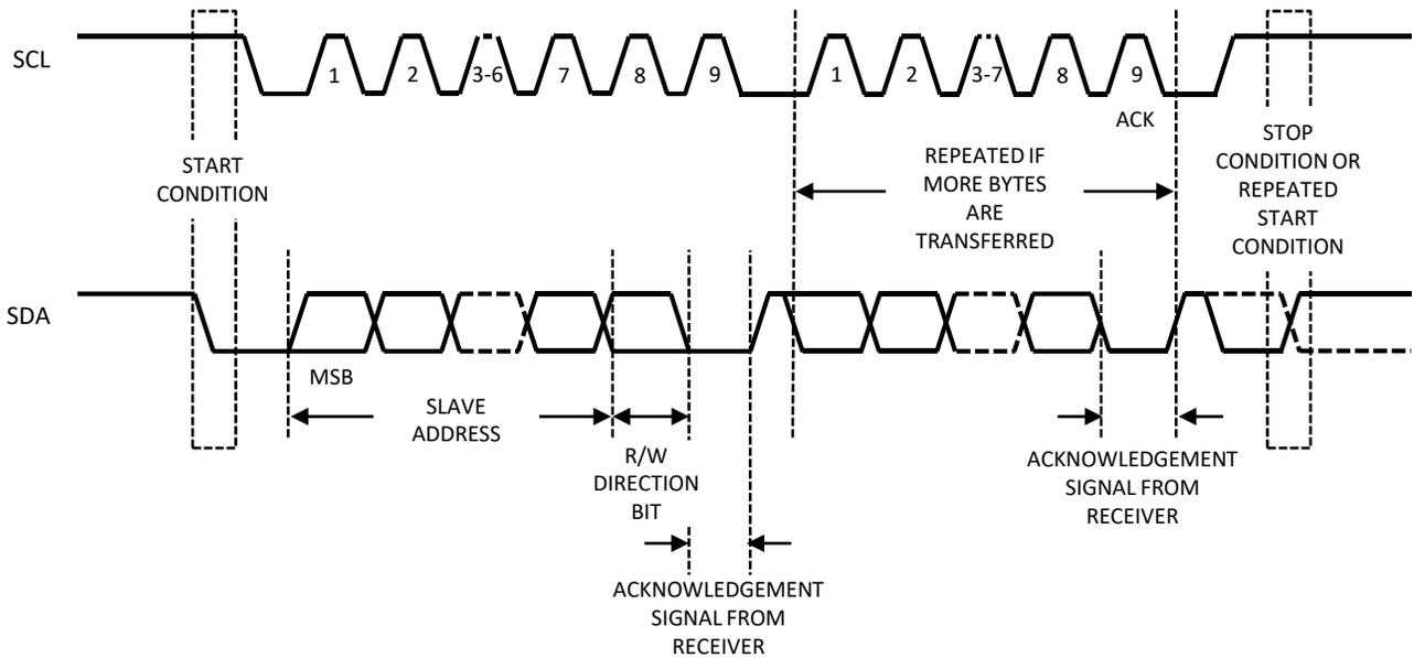
**Figure 6. Data Transfer on I<sup>2</sup>C Serial Bus**
