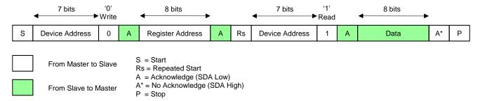
Figure 8. I<sup>2</sup>C Read Cycle
