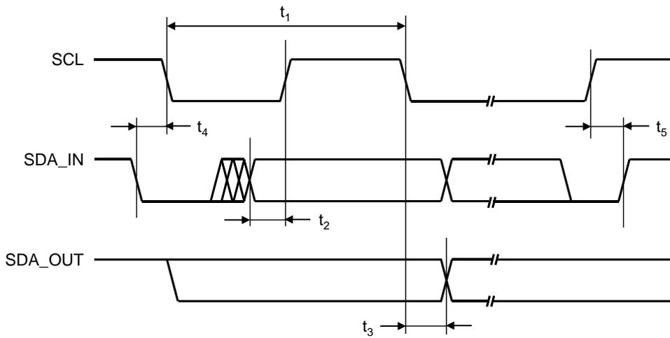
**Figure 1. I<sup>2</sup>C Compatible Interface Timing**
