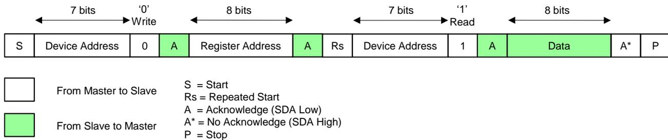
**Figure 8. I<sup>2</sup>C Read Cycle**
