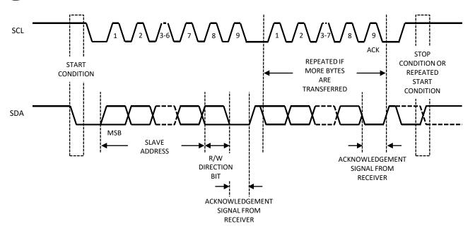
Figure 6. Data Transfer on I<sup>2</sup>C Serial Bus
