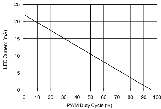
Figure 6. RC Filtered PWM Dimming Linearity (1kHz)
