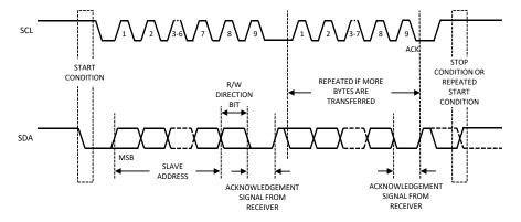
Figure 2. Data Transfer on I<sup>2</sup>C Serial Bus
