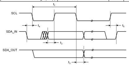
Figure 1. I<sup>2</sup>C Compatible Interface Timing Diagram
