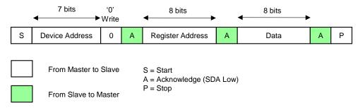
Figure 3. I<sup>2</sup>C Write Cycle
