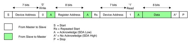
Figure 4. I<sup>2</sup>C Read Cycle
