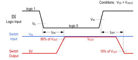
Figure 2. Switch Enable/Disable (via EN falling/rising) Timing Diagram
