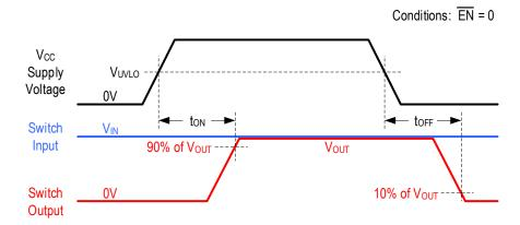
Figure 1. Switch Enable/Disable (via V<sub>CC</sub> rising/falling) Timing Diagram
