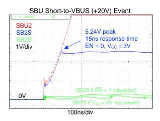
Conditions: SBU2 =  $25m\Omega$  short to +20V SB2S (SB2S) = open, no load
