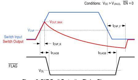
Figure 3. OVP Fault Protection Timing Diagram
