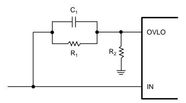
Figure 2. External OVLO Set Circuit
