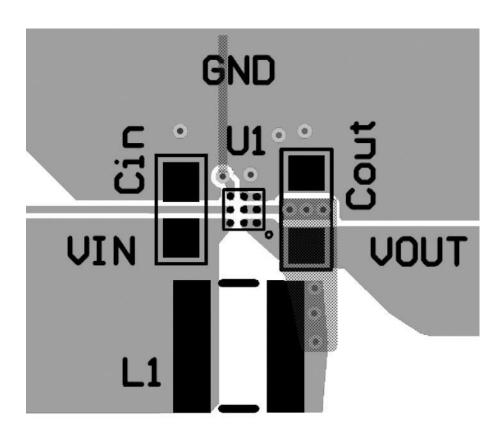
Figure 1. Recommended PCB Layout
