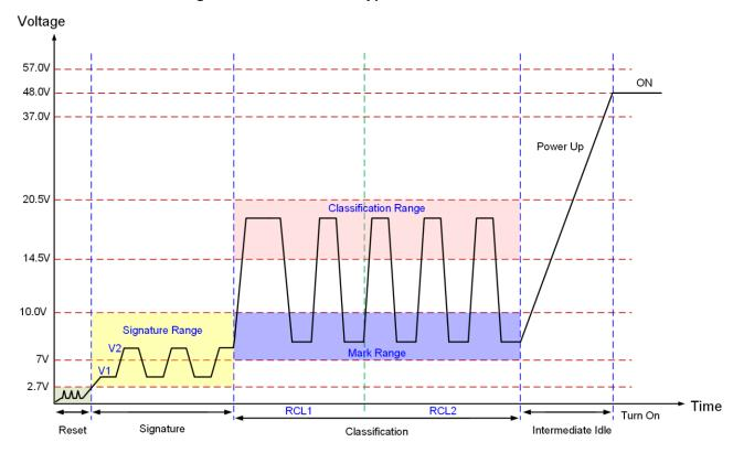
Figure 3. IEEE 802.3bt Typical Power-On Waveform
