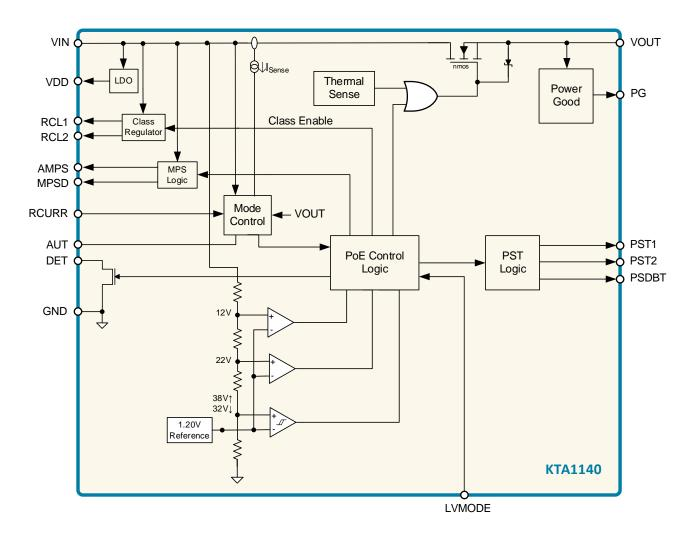
Figure 1. KTA1140 Block Diagram
