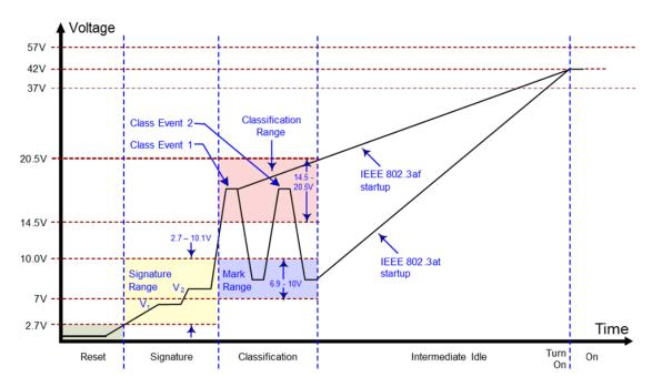
Figure 2. IEEE 802.3af/at Typical Power-On Waveform
