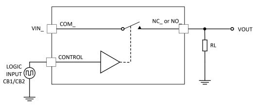
Figure 2b. Switch Timing Test Circuit
