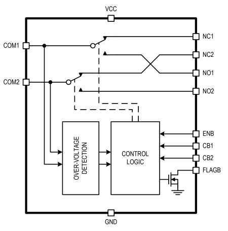
Figure 4. Functional Block Diagram
