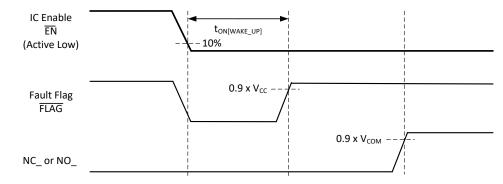
Figure 3. IC Wake-Up Timing Diagram
