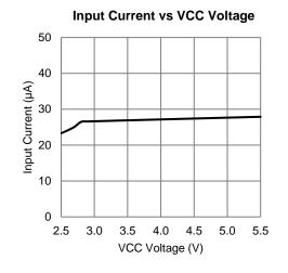
VCC = 3V,  $C_{VCC}$  = 1µF,  $T_{AMB}$  = 25°C unless otherwise specified.
