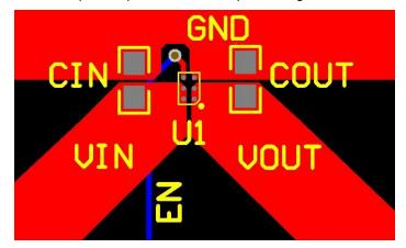
Figure 2. Recommended Layout for WLCSP-6 Package
